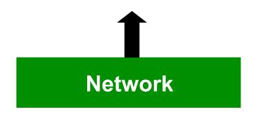
Taps network link passively, sends up a copy of all network traffic.
